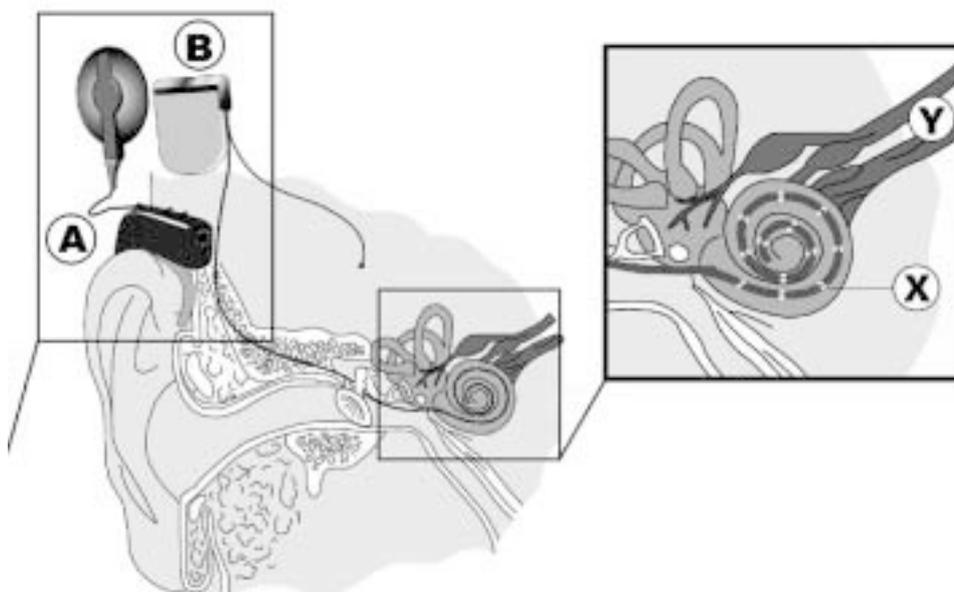
**Fig. 2.** Scheme drawing of the cochlear implant system: A — speech processor; B — implant; X — active electrodes; Y — auditory nerve
