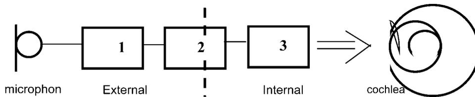
**Fig. 1.** Components of cochlear implant systems: 1— speech processor, 2 — transcutaneous transmission link, 3 — implanted receiver, decoder and stimulator in the same housing
