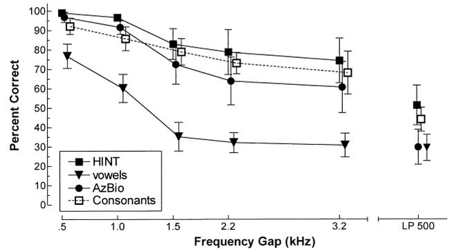
Fig. 2. Speech understanding as a function of frequency gap. The parameter is type of speech material.
