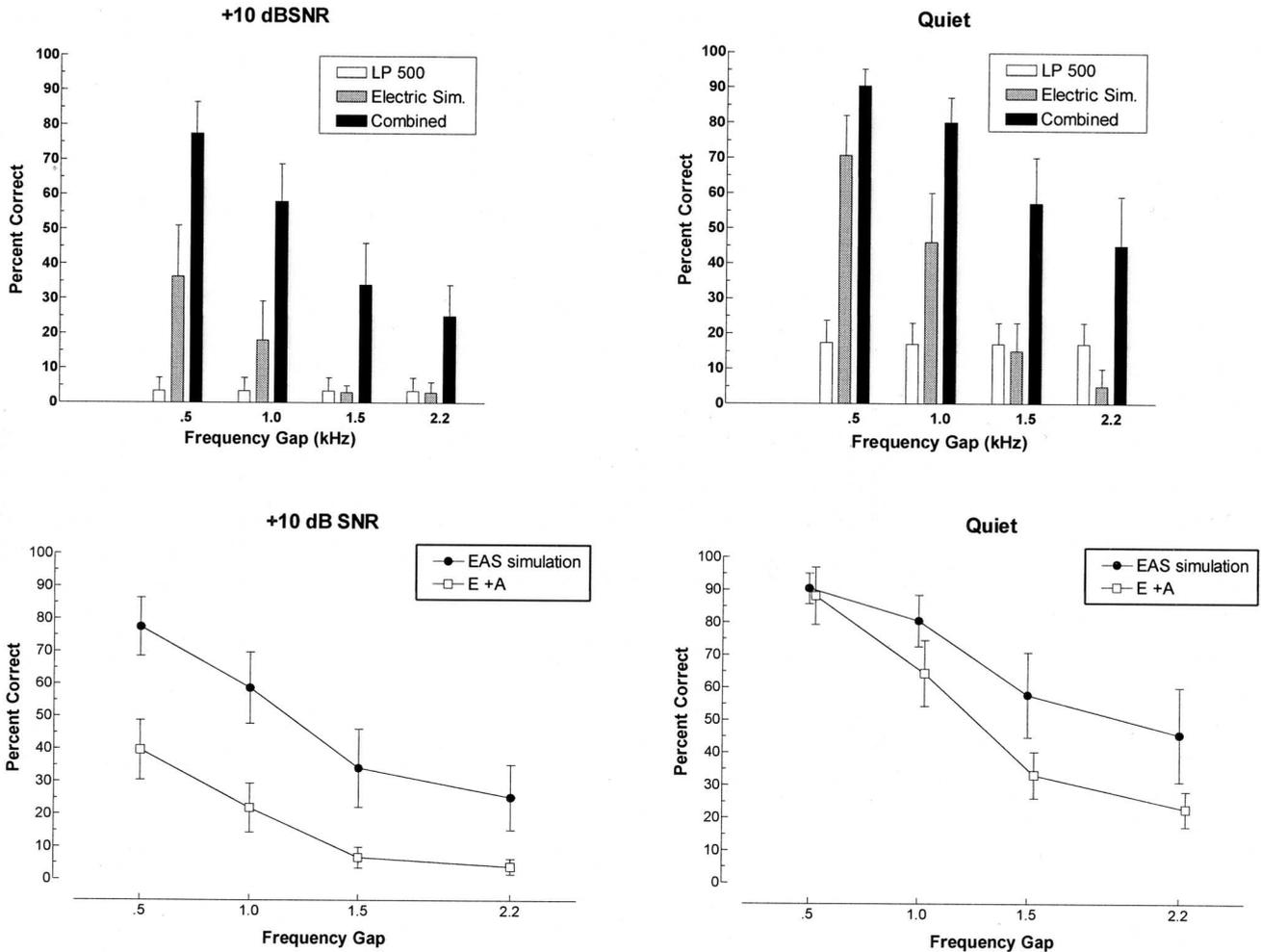
Fig. 5. Top, Percent correct scores in noise and quiet as a function of frequency gap for (1) signals low-pass-filtered at 500 Hz, (2) for simulations of electrical stimulation, and (3) for simulations of EAS. Bottom, percent correct scores in noise and quiet as a function of frequency gap for a simulation of EAS and for the sum of scores from the acoustic-only and simulated electric-only conditions.
