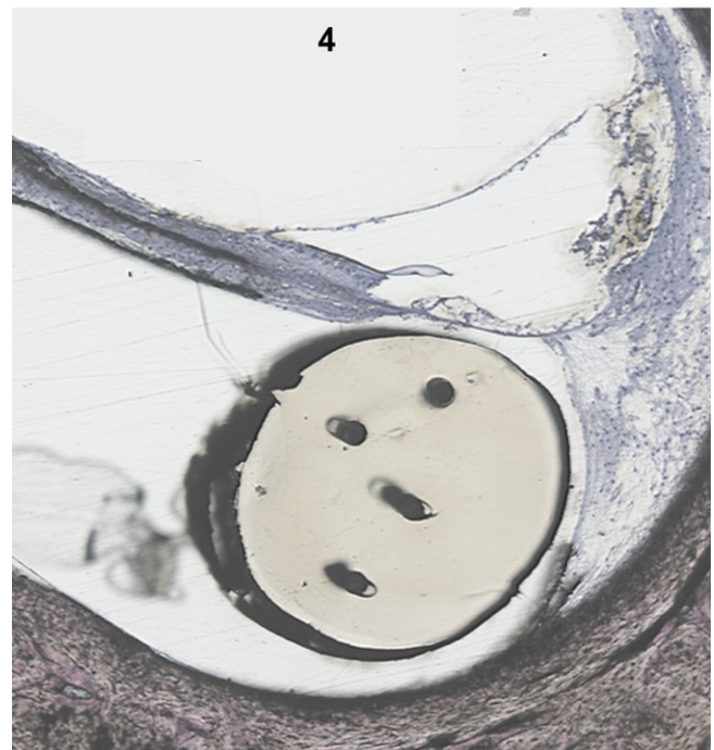
Fig. 3 and 4. Cochlear implant electrode in situ, in distance to the basilar membrane (BM) (Fig. 3), and in close contact – uplifting the basilar membrane (Fig. 4).
