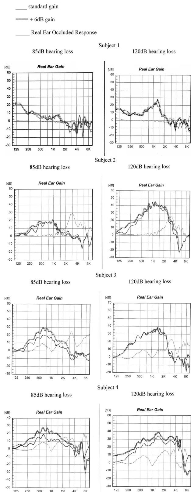
**Fig. 2.** The real ear insertion gain measurements for each subject and each hearing aid fitting are shown on the graphs. The single dark line indicates real ear gain for the standard hearing aid fitting. The double line shows the hearing aid fitting measurement with an additional gain of 6 dB. The real ear occluded response is shown by the lighter single line.
